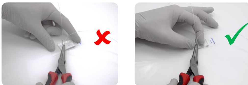
Figure 18: Diagram showing improper (left) and proper (right) grip of the vivoChip-2x while removing the metal coupler from the inlet or exit
