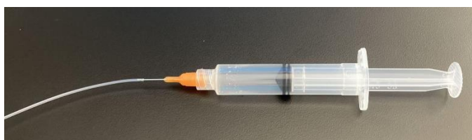
Figure 10: Photo of the luer stub screwed onto the 5 mL syringe
